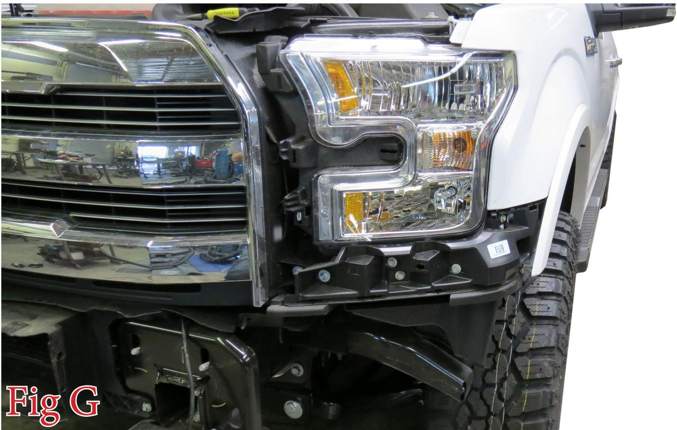
9. Remove the three bolts referenced in (Fig H) that were sitting behind the headlight bezel. Then, pull the air dam down and off the vehicle.
