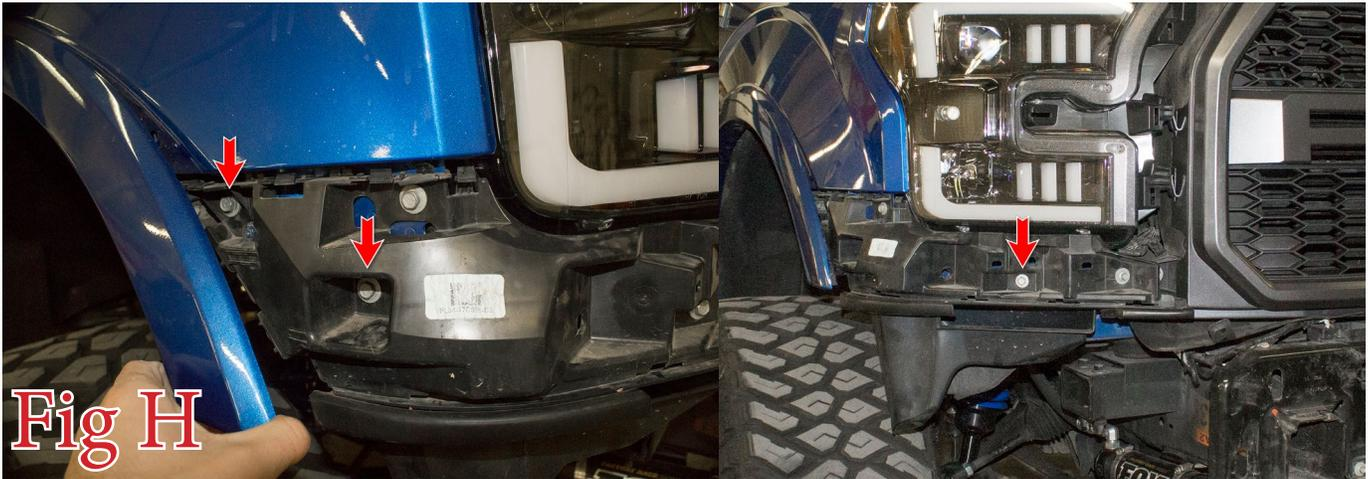
10. Push the headlight bezel back onto the vehicle and reinstall the plastic clip that was removed in Step 5. Then, push the fender flare back into place and reinstall the 7mm bolts you removed in Step 6.
