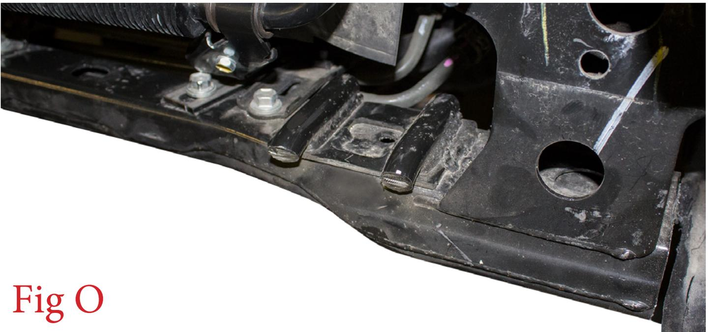
17. Using a 17mm Socket, remove the lower cross member mounting bolts (x4). Then, remove these cross members. **Save two of these bolts for reuse.** (Fig P)
