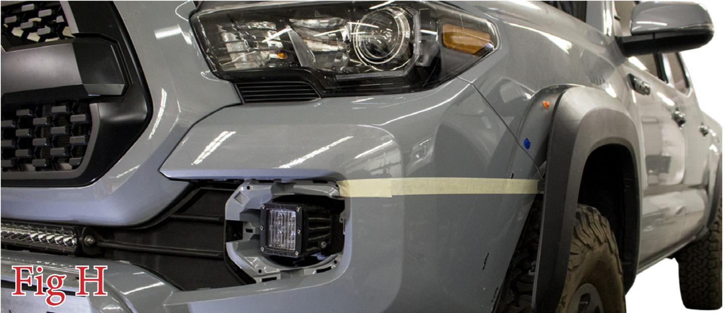
10. When you cut this line, leave about 1/4" of material to ensure you do not cut off too much material. (Fig I)
