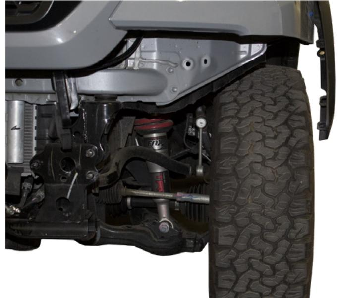
22. Use a utility knife (or something similar) to trim the two black plastic pieces just above the vehicle's frame horns as shown in (Fig V).
