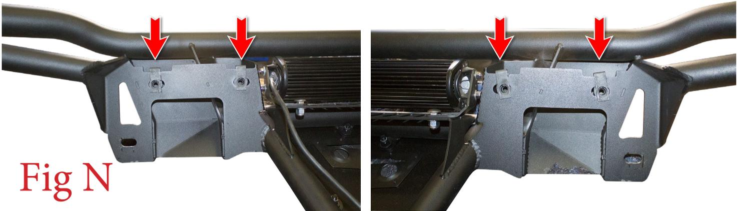
16. Set the bumper in place on the vehicle. Line the mounting holes on the bumper up with the mounting holes on the vehicle's frame horns. Then, install the supplied 3/8" Hex Head Bolts (x4) and 3/8" Fender Washers (x4) into the top mounting holes from the back side of the frame horns. Install the supplied 1/2" Button Head Bolts (x2), 1/2" Washers (x4), and 1/2" Lock Nuts (x2) into the lower mounting holes on the frame horns. Leave these bolts loose for now. (Fig O)
