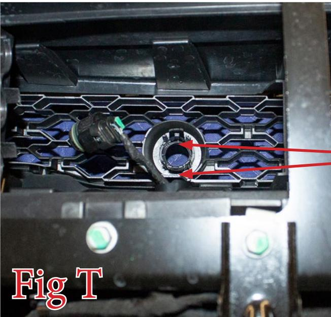
Squeeze these two tabs to release the mounting rings from the bumper
