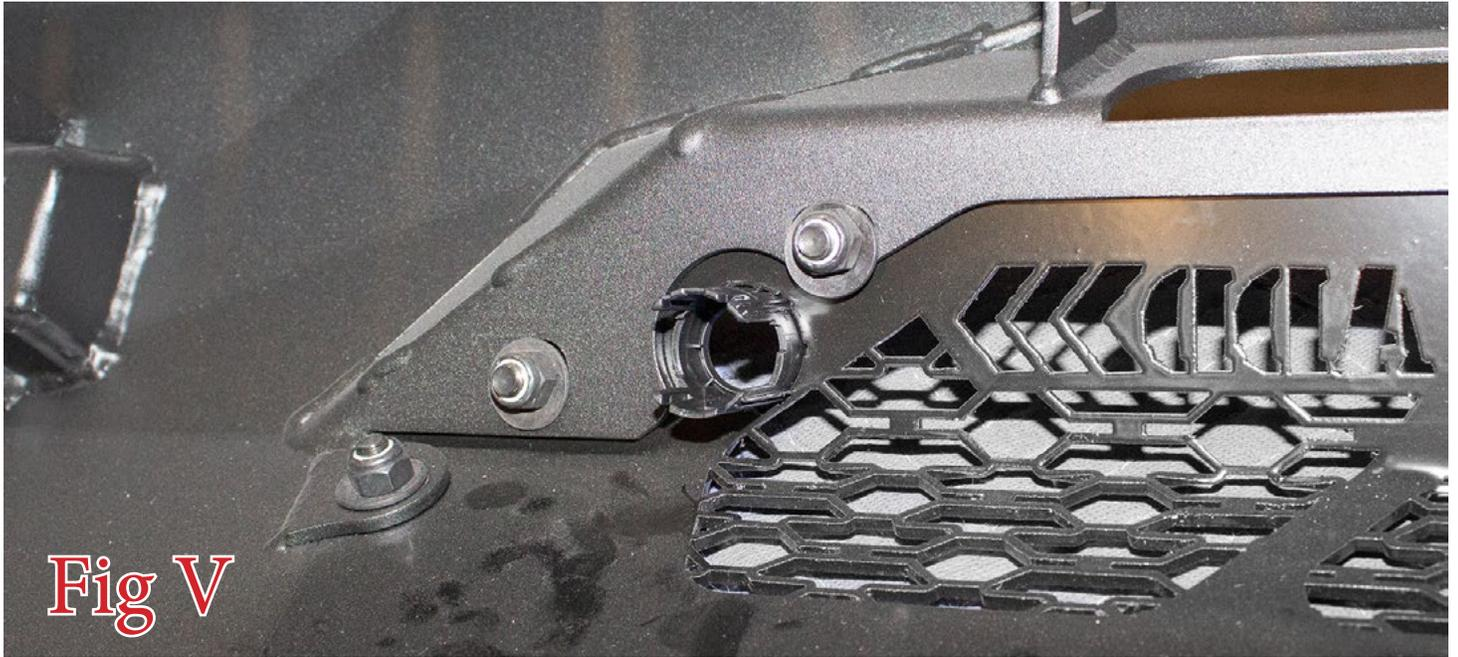
23. On the two outer sensor locations install the sensors in the provided bezels with the skinny side facing up. You will notice that one side will be oriented the same as factory and the driver side will be 180 degrees opposite. **\*\*Also note that the sensor plug needs to be 90 degrees to the ground\*\*** If your sensor bezel is loose in the bumper and can easily be rotated we recommend applying a small dab of silicone or epoxy to the back side to prevent them from rotating.
