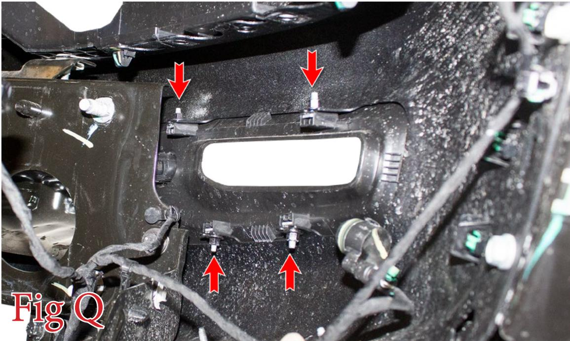
18. Use a 10mm Socket to remove the four bolts that hold the plastic trim piece to the edge of the OEM bumper. Then, remove that piece and use a Phillip's Head Screwdriver to remove the two marker light mounting screws. Remove the marker lights from the bumper. (Fig R)
