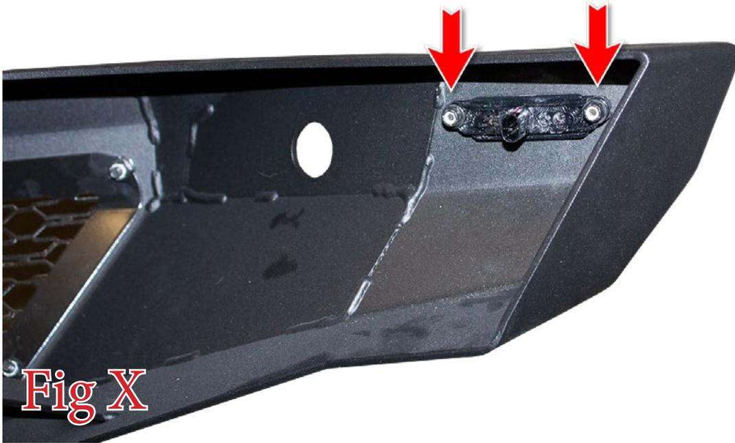
25. Install your light bar and cube lights now. For the light bar, use the supplied light mount kit. The installation instructions for that kit can be found here:
