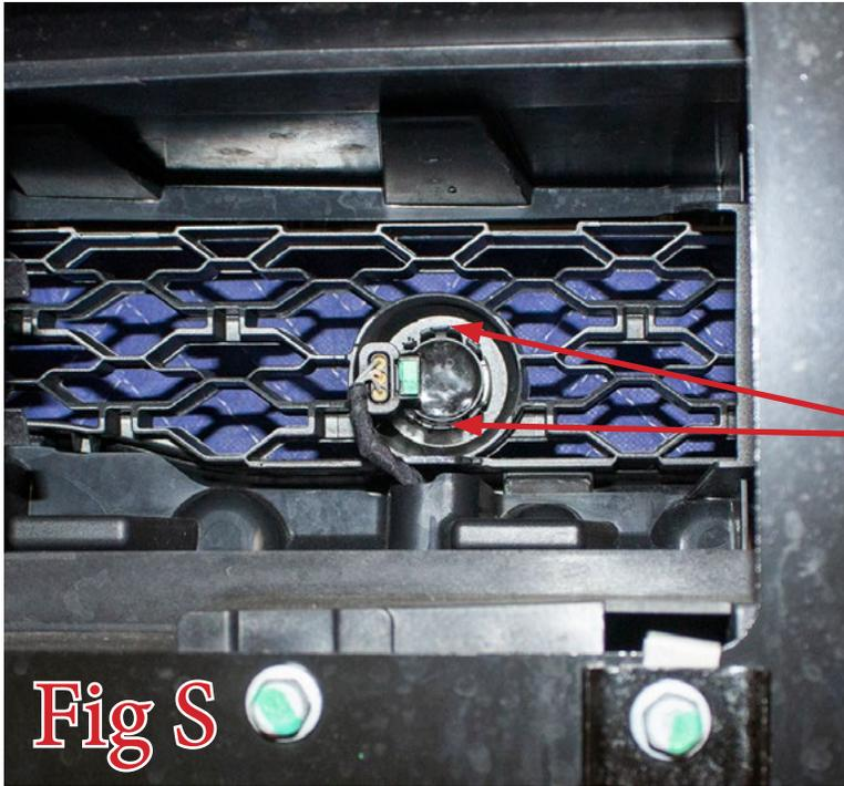
Spread these two tabs to release the parking sensor from its mounting ring
