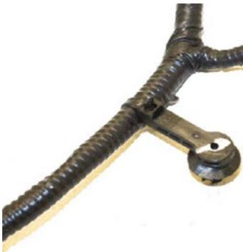
Strip back the wire loom starting at this connector and ending at the main harness connector so it looks like below when you are complete.
