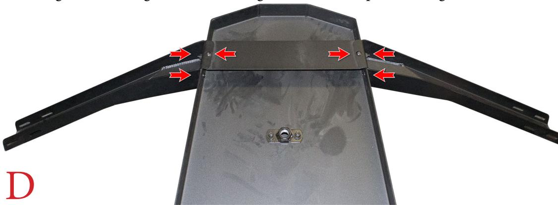
5. Find one of the tire carrier mounting pieces. Set it in place, then secure it loosely by installing the supplied 3/8" Bolts (x10), 3/8" Washers (x10), and 3/8" Lock Nuts (x10). (Fig E) We do not recommend installing the second mounting piece until the tire carrier portion is being installed on the truck.
