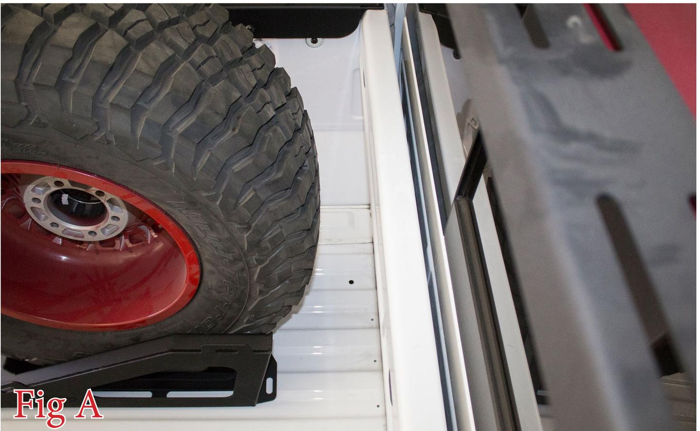
2. With the tire carrier placed how you want it, make a mark at each of the 4 mounting holes you would like to use. Make sure the the mounting holes you use line up with the raised parts of the truck bed so that the bed sits flush with tire carrier where its bolted down. (Fig B)
