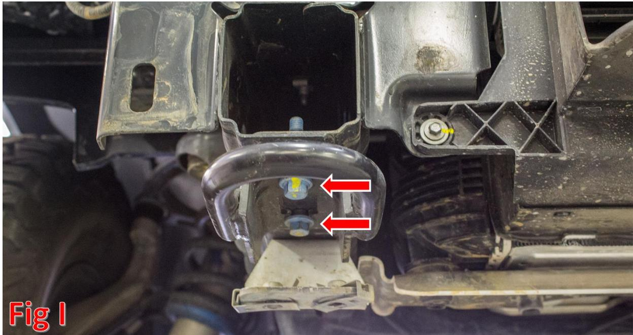
10. Remove each of the Skid Plate Brackets by removing the 13mm bolt that holds each of them on. There is one bolt per side. (Fig J)
