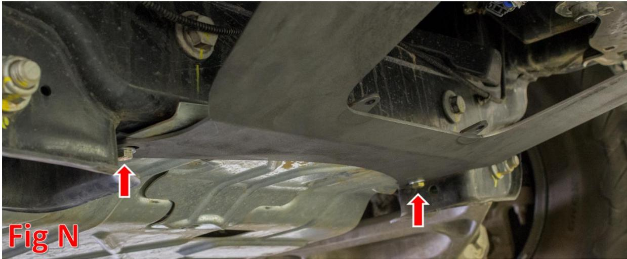
5. Line up the bumper so that it is straight in relation to the grill/headlight bezels. You may need one person to hold the bumper in place while another person tightens the bolts.
