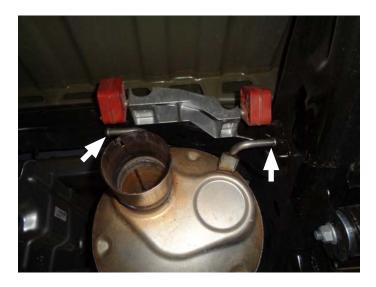
6. Disassemble nuts (x2) from factory pipe and catalytic converter flange. Remove muffler and factory pipe from vehicle.
