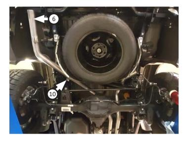
15. Place **clamp (10)** onto **right exit pipe (7)** then connect it to right overaxle pipe. Insert wire hanger into isolator then tighten clamp just enough to allow for adjustment.
