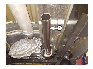
10. Fasten inlet with (x2 ea) bolts (9), flat washers (11), lock washers (12) and nuts (10). Place clamp (8) onto extension (2) and connect it to inlet pipe. Insert hanger in isolator then tighten clamp to allow for adjustment.
