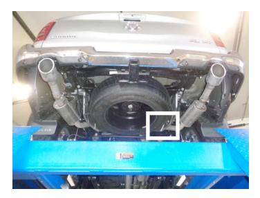
4. Remove factory tailpipe from vehicle by cutting it near muffler outlet and dismounting wire hangers from factory mounts.
