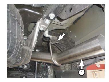
13. Connect **left overaxle pipe (5)** to muffler and hang wire hanger in stock isolator. Tighten clamp just enough to allow for adjustment.
