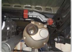
5. Remove factory muffler wire hangers (x3) from factory isolators and detach grounding wire.
