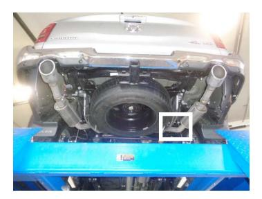
4. Remove factory tailpipe from vehicle by cutting it near muffler outlet and dismounting wire hangers from factory mounts. Remove and retain tailpipe isolators for later use.
