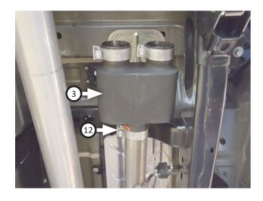
12. Route **right front (4)** and **left front (5) tailpipes** over axle then connect them to muffler. Insert their wire hangers into isolators then tighten clamps just enough to allow for adjustment.
