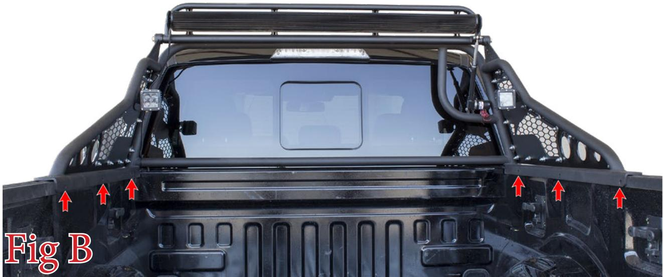
3. Line the mounting holes on the chase rack up with the newly drilled mounting holes on the bed rail. Then, use the supplied 1/2" Bolts (x6), 1/2" Washers (x12), Backing Plates (x6), and 1/2" Lock Nuts (x8). Mount the hardware exactly as shown in (Fig C). Once all bolts are loosely installed, torque the mounting bolts to 70 foot pounds.
