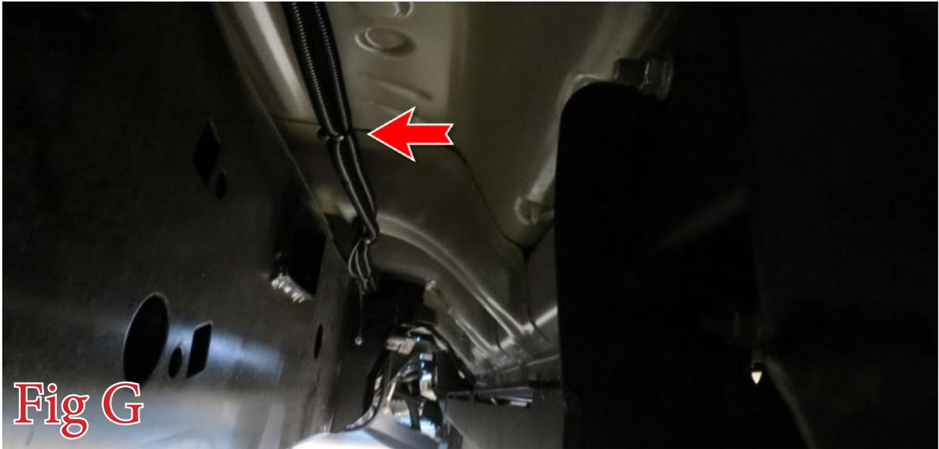
10. Send the two red wires with blue butt connectors (for the 50" and the other is unused), the green wire (for the light's backglow), and black wire with an eyelet (for ground) forward into the engine bay on the passenger side.
